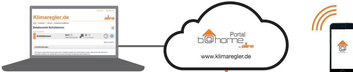
Control and monitoring of heating/cooling regulation from anywhere at anytime via the LAN/WLAN (no Internet connection required)
