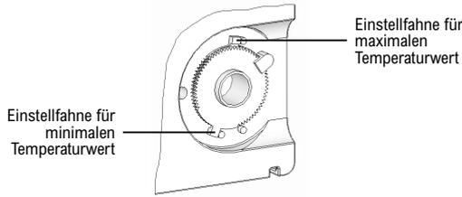
The setting pins located underneath of the adjusting knob enable to delimit the setting range of the controller mechanically. To enable this, the adjusting knob must be removed by pulling it off and, after the adjustment of the related pins (end stops, red for max. and blue for min. setting) be put on again in order to lock the limitations.
